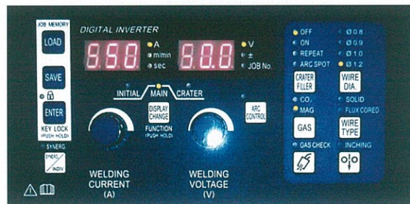
Figure 2 : one knob switch to wire speed display
